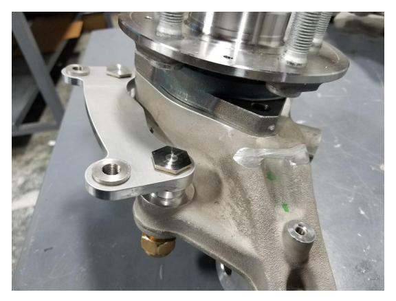
\*Locate the brackets provided in the kit along with the caliper bracket mounting bolt kit (4x 9/16 hex head with nylocs and split rings). Clean bolts with acetone to remove any oil. Using the factory ear locations, you will mount the bracket on top of the ear location. Using the spacer provided in between the bracket and the spindle ear and the 9/16 washer between the nut and ear. Use red Loctite to lock it in place and Torque to 50 ft. lbs.
