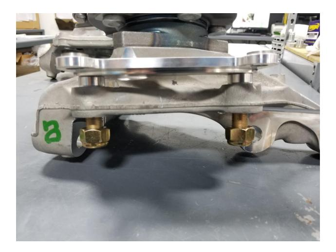
\*Bolt rotors to hats using the 5/16 -18 ¾ low head screws. Make sure to clean bolts with acetone and use red Loctite to secure. The hat should be mounted on the flat side of the rotor.
