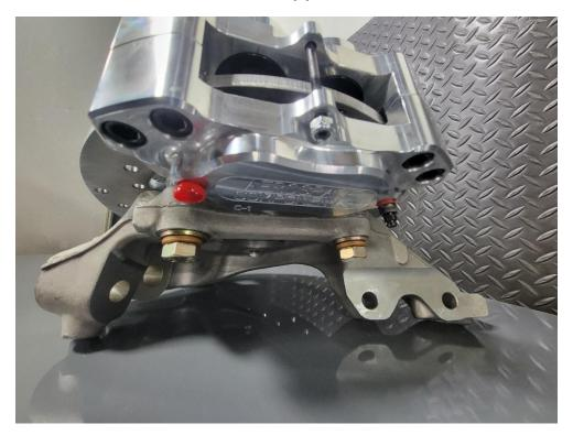
\*Drop the pads into the calipers with the friction side facing the rotor and secure them with the pad retaining bolt and nyloc nut. Be sure the bolt extends through the locking feature of the nut. Make sure the brake pads are the only thing touching the rotor and that the rotor spins freely.
